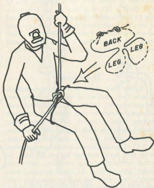
Figure 2. A snaplink rappel rig for steep slopes. Inset illustrates seat sling.
